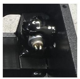
7. Apply high strength Loctite to the 1/4-20 AUX hole cap screw. Dab any excess Loctite with a paper towel, if necessary.
