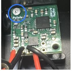
10. Guide the LED wires into the corner near the  $\frac{1}{4}$ -20 thread.
