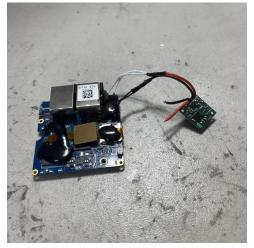
If you are assembling the UPS variant, solder the two flying lead input wires you prepared earlier on the NanoPi R2S Plus to the UPS's *UPS* annular rings (on the frontside) instead.
