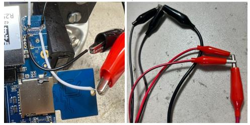
e. Verify full boot after waiting 30 seconds. With an external device attached, you can verify your computer's connection by referencing the SMD status light labeled *LAN*, which should illuminate solid green.
