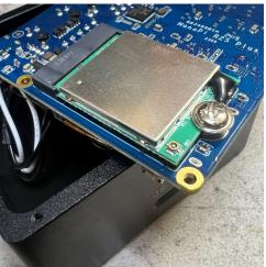
19. Connect the I-PEX MHF4 connector to the M.2 HaLow module.
