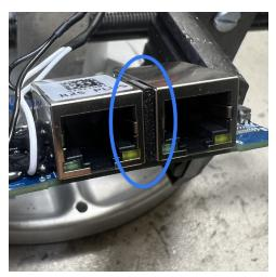
2. Align <u>RJ45 Gap Spacer Two</u> adjacent to the *LAN* port with the textured side exposed; hot glue into place.
