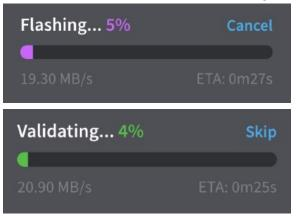
Heads up! If this process takes two minutes per step (i.e. four minutes total), you likely have a bad eMMC module and it will not function properly to run the OS for TeeHee HaLow. Please replace it before proceeding.
