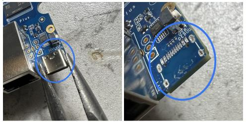
4. Chemically remove the horizontal USB-C port labeled 5V IN & DATA.
