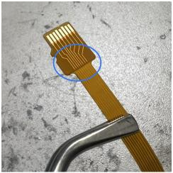
2. On the male dummy end of the ribbon cable, use a needle nose pliers to hold the rigid plastic while applying even lateral pressure across the ribbon to gently peel back 3mm from the plastic stencil.
