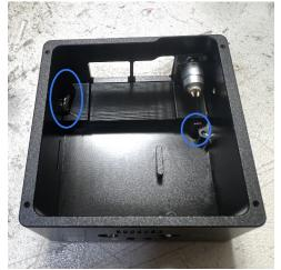
6. Encapsulate the Lemo OB 2-Pin chassis connector in hot glue to prevent loosening over time. Ensure the solder cups of the connector and the multipurpose button hole remain exposed and accessible.
