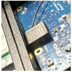
23. Attach the lid using the four black 0-80 screws. Secure the two screws on the RJ45 side first.
