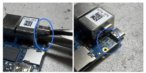
2. With a needle nose pliers and flush cutter, physically remove the horizontal USB-A port labeled USB 2.0.
