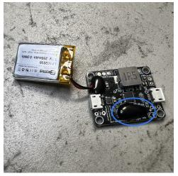
6. Hot glue the <u>UPS Insulator</u> to the bottom to electrically isolate the exposed solder joints.
