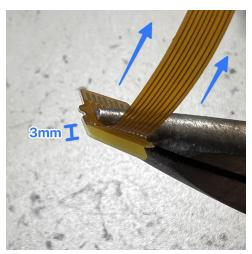
3. Use a flush cutter to remove 2mm of plastic from the rear edge of the male end plastic dummy unit that you just delaminated.
