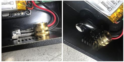
15. UPS variant only: Hot glue the UPS battery into the corner adjacent to the Pololu buck converter.
