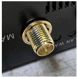
c. Apply high strength Loctite to 1mm of the exposed RP-SMA threads closest to the chassis. Dab any excess Loctite with a paper towel, if necessary.
