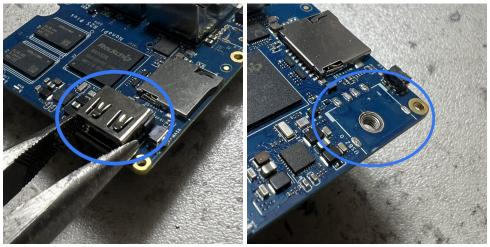
3. With a needle nose pliers and flush cutter, physically remove the horizontal USB-C port labeled USB DEBUG.
