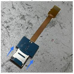
2. Using the flat end of a nylon probe, insert the prepared dummy Micro SD male end into the NanoPi R2S Plus Micro SD card slot, ensuring it "clicks" into place.
