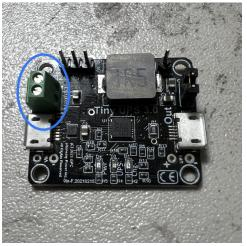
3. Connect the two *On-Off* annular rings with a solder bridge.
