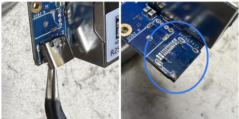
d. Using an ESD cleaning brush, gently scrub 90%+ isopropyl alcohol over the SMD pads once the port has been fully removed. Allow time to air dry or dab dry with an ESD polyester wipe.
