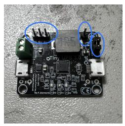
2. Desolder the battery input screw-down terminals and wick away any excess solder from the *Battery* annular rings.
