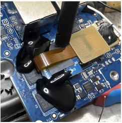
13. Once the hot glue has dried, disconnect the rubber-coated alligator clip that secured the eMMC module.
