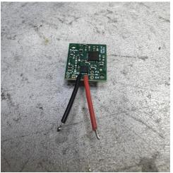
If you're assembling the UPS variant: Also solder <u>30mm ground and positive wires</u> from the Pololu buck converter output backside (the side without cylindrical capacitors) to the UPS's *Vin* annular rings on the frontside (the side with the 1R5 inductor).
