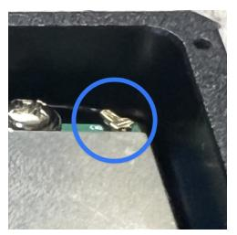
20. Insert the NanoPi R2S Plus into the chassis, RJ45 ports first. Guide the RP-SMA extension cable through the crescent gap on the side of the NanoPi R2S Plus while ensuring no wires get pinched.
